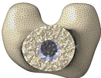
Fig. 5 - Consistent mesh quality in non-manifold assemblies
